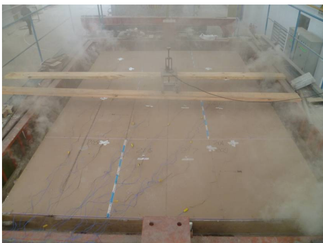
Photo 27: The unexposed surface of the specimen after a test duration of 90 minutes.
